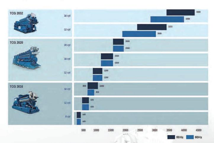
MWM's product portfolio comprises gas engines and gensets in the output range from 400 kWel to 4,500 kWel. In this way, it is possible to set up power plants with an output of up to 100,000 kWel and more.
